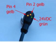
Pin 4: Differential pressure switch has tripped Pin 2: Differential pressure switch O.K.
